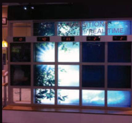
As this demonstration at Greenbuild 2011 shows, SageGlass electronically tintable glass from Sage Electrochromics allows users to select preset tint levels between the low and high ends of the glass's dynamic range.
