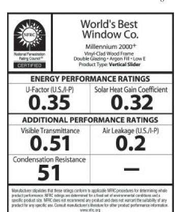
Figure 11. The NFRC label discloses performance factors for each individual window. Visible transmittance, air leakage, U-factor, and solar heat gain coefficient (SHGC) ratings all enable determination for an optimal window performance choice. Learn more about the NFRC label at http://www.nfrc.org/label.aspx.
